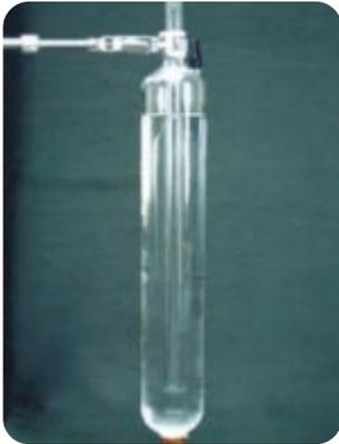
Triple point of water cell used on the ground for ITS-90 calibrations
